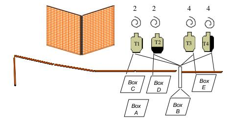
**SETUP NOTES**: T1-T2 are double exposure targets. T3-T4 are quad exposure. Align steel in a row opposite of each other.
